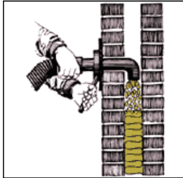
Figure 18 Insulation injected into a hollow wall (23).
