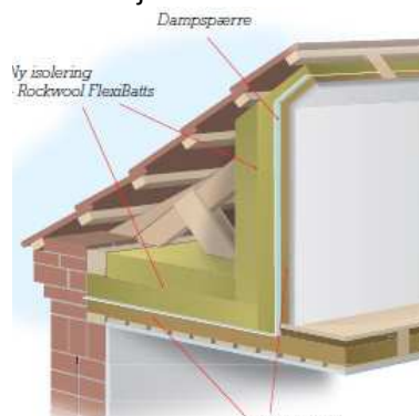
Figure 27 Re-insulation of the attic below the slanting roof (23).
