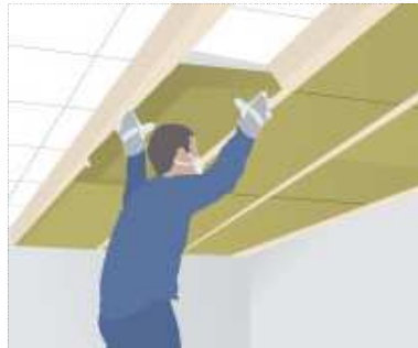
Figure 24 Re-insulation underneath horizontal division (23).
