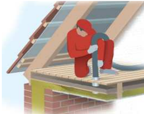
Figure 22 Insulation injected into a horizontal division (23).
