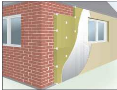
Figure 19 External re-insulation of the facade (23).
